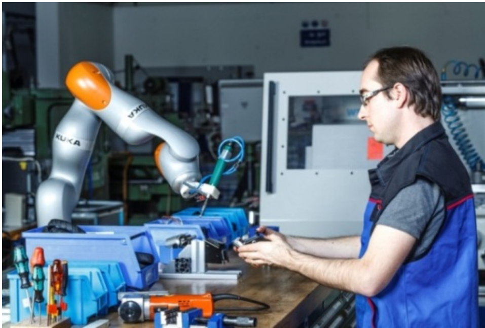
Lightweight portable robot as physical assistant
