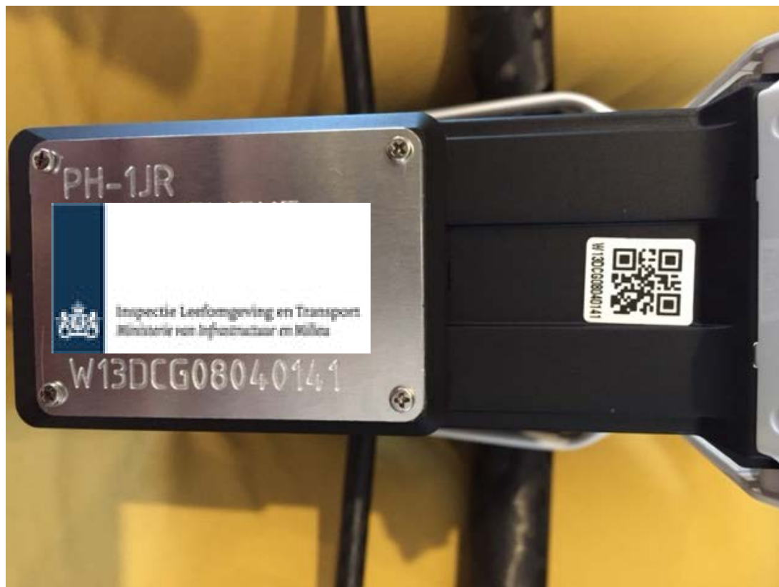
Register : PH-1JR - DJI Inspire 1 Fire Resistant Plate
